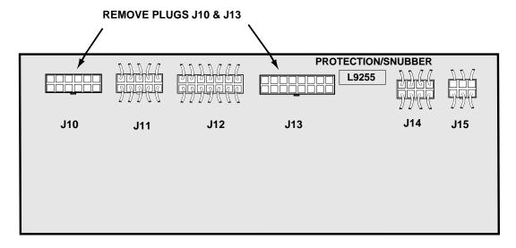
FIGURE F.11 - PROTECTION BOARD PLUG LOCATIONS
